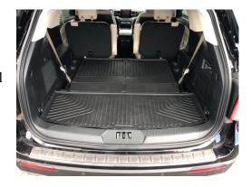
4. The first time the rear seat backs are moved to the upright position, move the seats slowly taking care to insure the accordion section of the liner folds outward as shown. This may need to be assisted from the backside.
