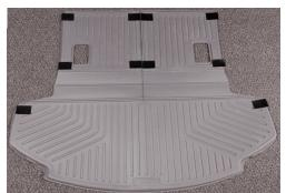
2. As boxed, the liner is not "split" to allow the 3<sup>rd</sup> row seat backs to fold independently. If you wish to have this functionality, the seat back portion can be split down the middle as shown in the photo. There is a trim groove molded in the center of the liner to guide trimming.
