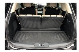
5. The liner at this point is fully installed and is ready to use. If the liner needs to be removed, grab the rectangular Velcro patches and hold them firmly in place as you pull the liner from the seat. This Velcro piece is intended to stay attached to the seat back and cargo floor to reduce ware from the liner being installed and reinstalled for cleaning.
